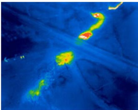
*A hot-water pipeline heats the surface of the ground and, therefore, can be detected by a thermal camera located on the drone. Using this camera, areas can be detected where the pipeline is broken or where the penetration of hot water heats up the affected earth.*
