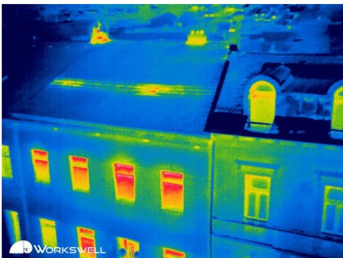
**Construction roof thermal bridges. They may be signs of serious roof damage and leaks.**
