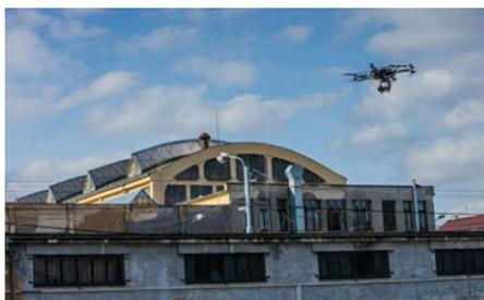
when inspecting roofs (where defects are the most common) it is very difficult to check the masonry using a manual thermal camera. A good solution is Workswell WIRIS thermal imaging system for drones, which is just as convenient as manual systems. Moreover, the system is calibrated and, therefore, the results of the measurements are conclusive.
