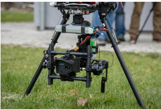
Thermal imaging camera Workswell WIRIS mounted on a drone
