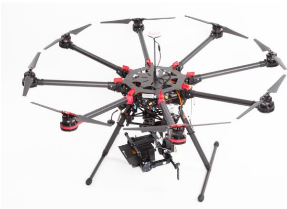
Thermal imaging camera Workswell WIRIS mounted on a drone
