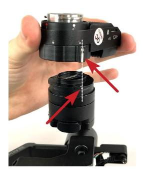
4. Secure the mount system between the gimbal and gPort
