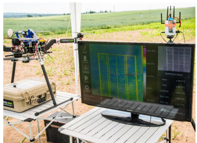
Ground station with Workswell WIRIS, LCD screen and second drone.
